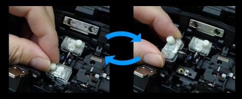
The transparent electrode covers support wider illumination of the v-groove. As the sheath clamp opens on the opposite side of the illumination lamp, the sheath clamp area is illuminated without shadow.
