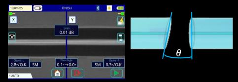
\*G.652 splicing result measured with a cut-back method. The splicing result changes depending on the fiber type and fiber characteristics.
