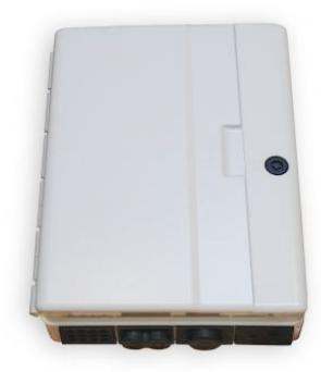
The housing is made of Polycarbonate plastic giving excellent mechanical strength at a very low weight. Metallic parts such as screws, microduct and cable holders etc. are made of stainless steel. The cable inlet seals and other rubber parts are of EPDM.
