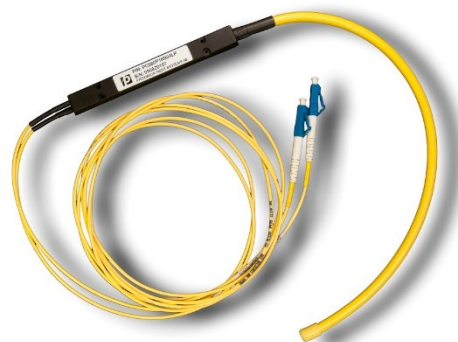
Figure 20 – FBG and circulator incorporated in a patch cord
