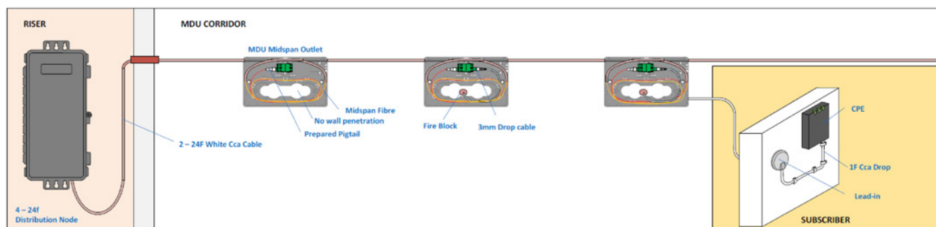
Installation layout of the discreet fiber system
