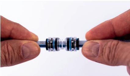
To disconnect the Microduct from the connector, make sure that the pressure in the system has been fully released before starting. First, remove the locking clamp. Then, press the collet towards the connector and pull out the Microduct.
