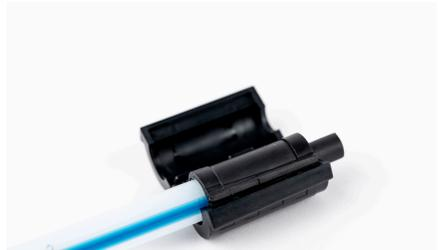
3. Close the housing, making sure that the seal is correctly positioned in the housing. Slide the entire component onto the pipe so that the end of the pipe abuts the seal on the inside, press firmly together and do not let go now. Attach the clamping rail to fix the divisible sealing element.
