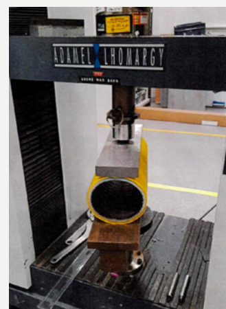
Figure 13. Pipe stiffness test setup.
