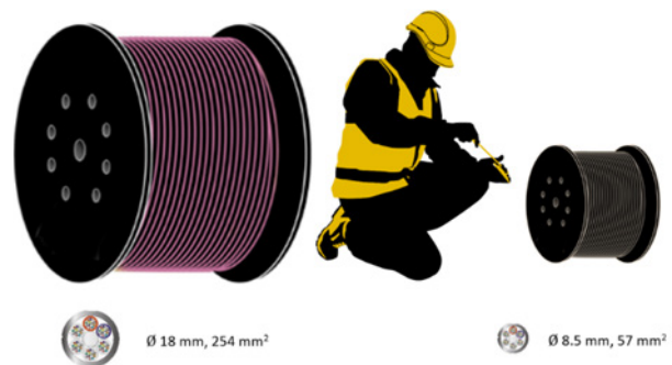
Figure 4. Comparison of drum handling of a reel for standard cable and micro cable.
