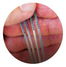
Hexatronic has a long experience in stripe marking of ribbons and with its unique production capabilities, stipe marking is the standard method to separate ribbons. This guideline will therefore only describe the preferred method 1.
