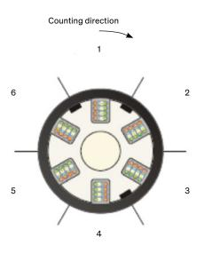
Slotted Core Profile, 8-fiber Ribbon, 8 to 192 Fibers
